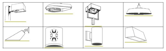
**Figure E:** Full cutoff fixtures are closed on top and mounted such that the bottom opening is horizontal. The mounting height and location may require additional shielding to prevent the lamp from being visible from any other property. A practical way to determine if a light fixture is a full cutoff fixture is that the lamp, any reflective surface or lens cover (clear or prismatic) is NOT visible when viewed from above or the side.
