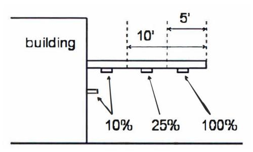
Figure K: Elevation view of a canopy or overhang attached
