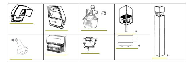
**Figure F:** This figure illustrates examples of fixtures that are NOT full cutoff fixtures. Note: Even though the lamps in these fixtures are shielded when viewed from the side or above, reflective surfaces within the fixtures or lens covers are directly visible from the side.
