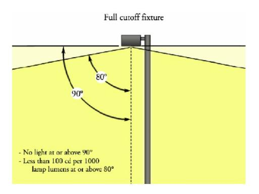
**Figure B:** Full cutoff fixtures do not allow any light to be emitted above the fixture.
