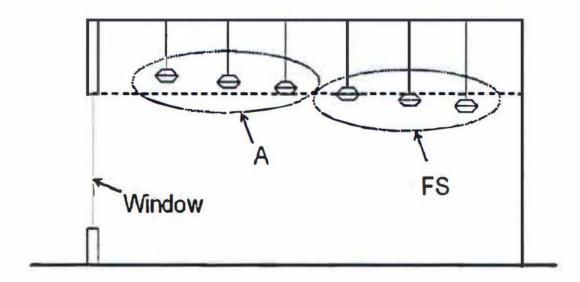
**Figure A:** Elevation view showing an application of indoor lighting, labeled 'FS,' which is subject to these requirements and indoor lighting, labeled 'A,' which is installed so that it is typically not subject to these requirements.
